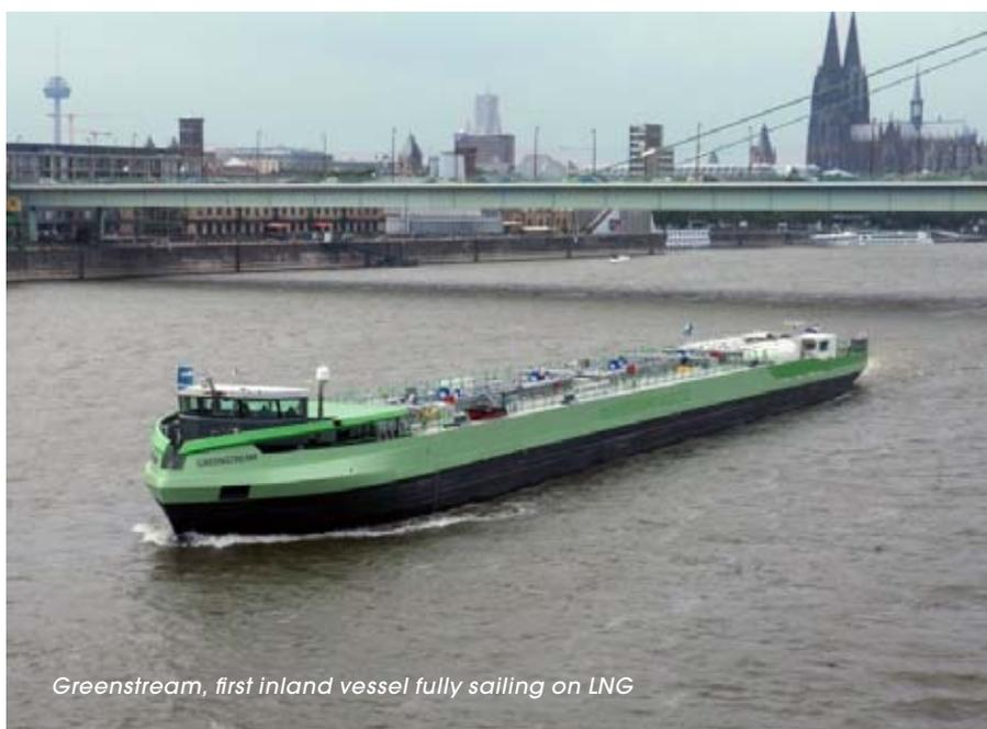
*Greenstream, first inland vessel fully sailing on LNG*
